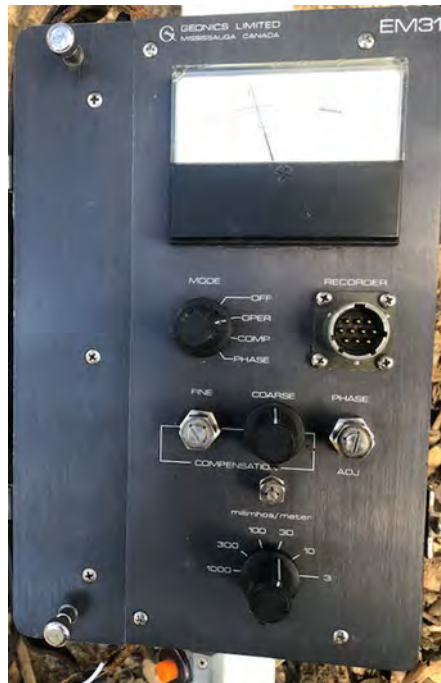
Figure 5.4. Picture of the EM-31 operating panel.
